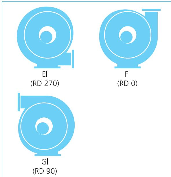
In the standard version, the equipment is supplied with the terminal box position 270° (top) and the cable inlet A (right). For explanations of the terminal box position and the cable inlet options, see page 14.
